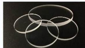
Fused Quartz discs are used for high temperature applications up to 1200°C (2192°F) or applications which require UV transparency.
