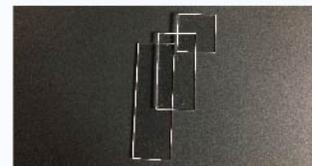
Fused Quartz microscope slides are used for high temperature applications up to 1200°C (2192°F) or microscopy applications which require UV transparency.
